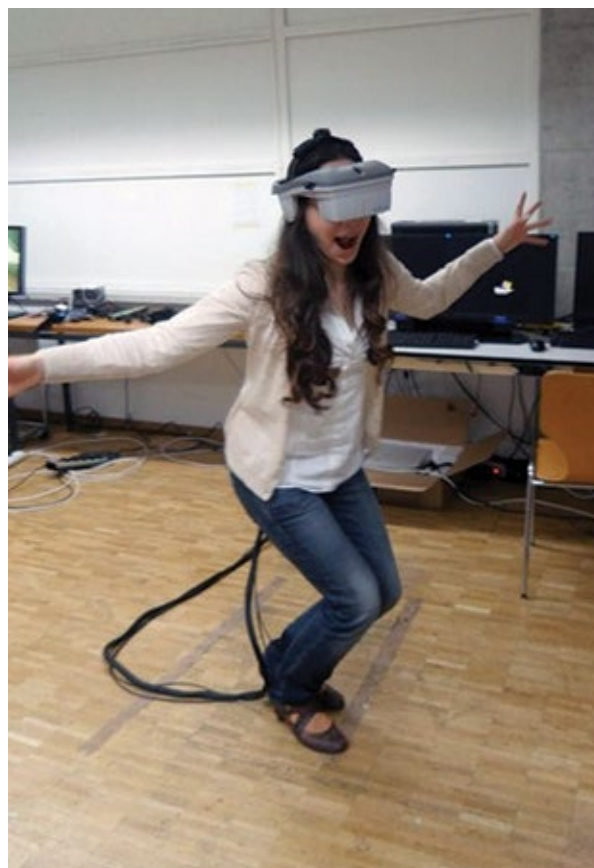
Virtual reality set-up for immersion in realistic scenes and interaction with avatars. The head mounted display is equipped for eye tracking.
