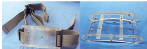
Acrylic calibration phantom.
