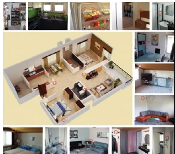
An example installation of the new assistive technology system in a two bedroom flat. Environmental data are acquired by sensors distributed in the rooms. The locations of the sensors are indicated with red circles.
