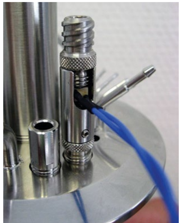
Autoclavable micro dosing unit on a mini bioreactor head plate.
