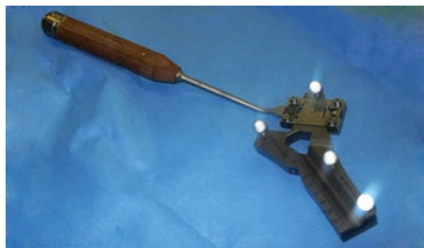
Navigated PAO chisel with calibration device.
