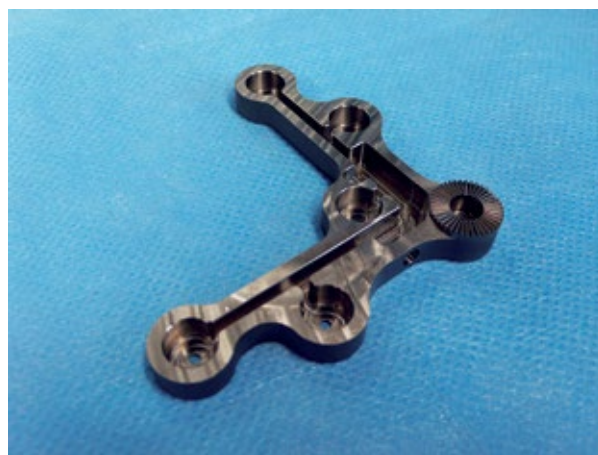
High accuracy tracking markers, constructed from titanium, allow measurement and control of a robotic system for minimally invasive cochlear implantation.
