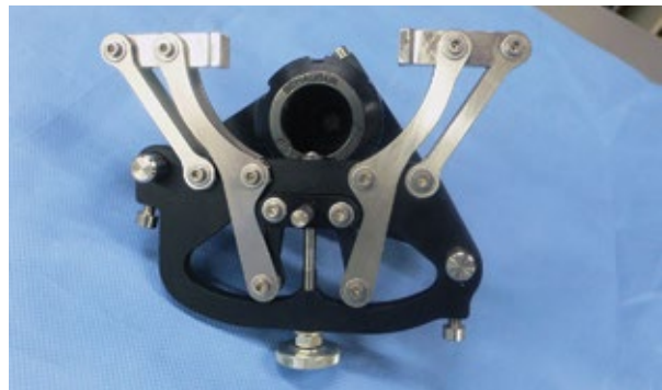
Custom extensometer clamp, constructed to ensure accurate fixation to thin bone samples.
