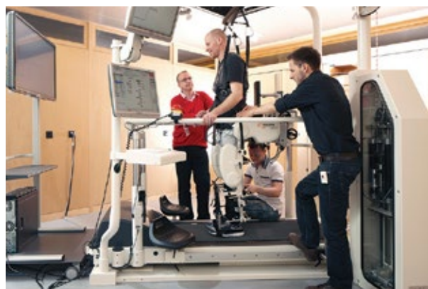
The IRPT's dedicated research lab within the Reha Rheinfelden: The Lokomat has been enhanced for cardiopulmonary rehabilitation of stroke patients.
