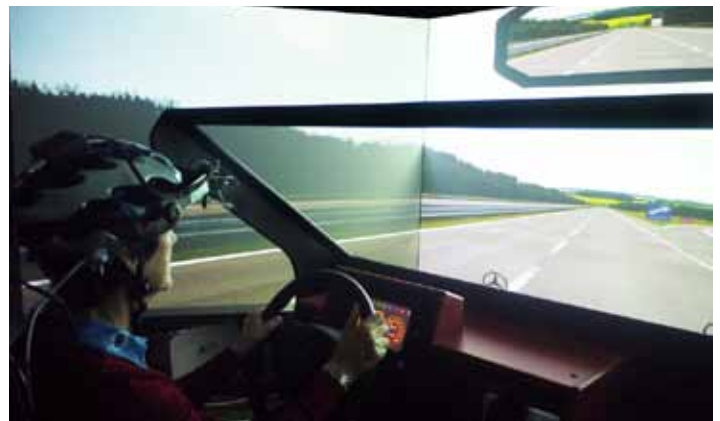
Test driving in a visual exploration experiment. The test subject wears a helmet with an integrated eye tracking camera to measure gaze direction.
