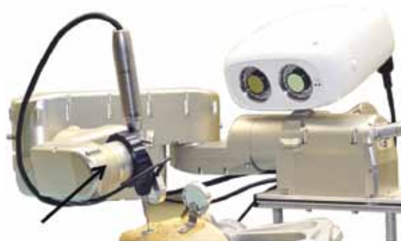
The robot system compensates for kinematic errors and deflections of its robotic arm as well as for patient movement by means of an optical tracking system with an accuracy of less than 20 microns.
