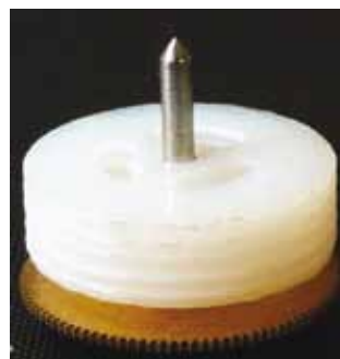
Prototype of a Tesla turbine (left) and numerical flow visualization between two turbine discs (right).
