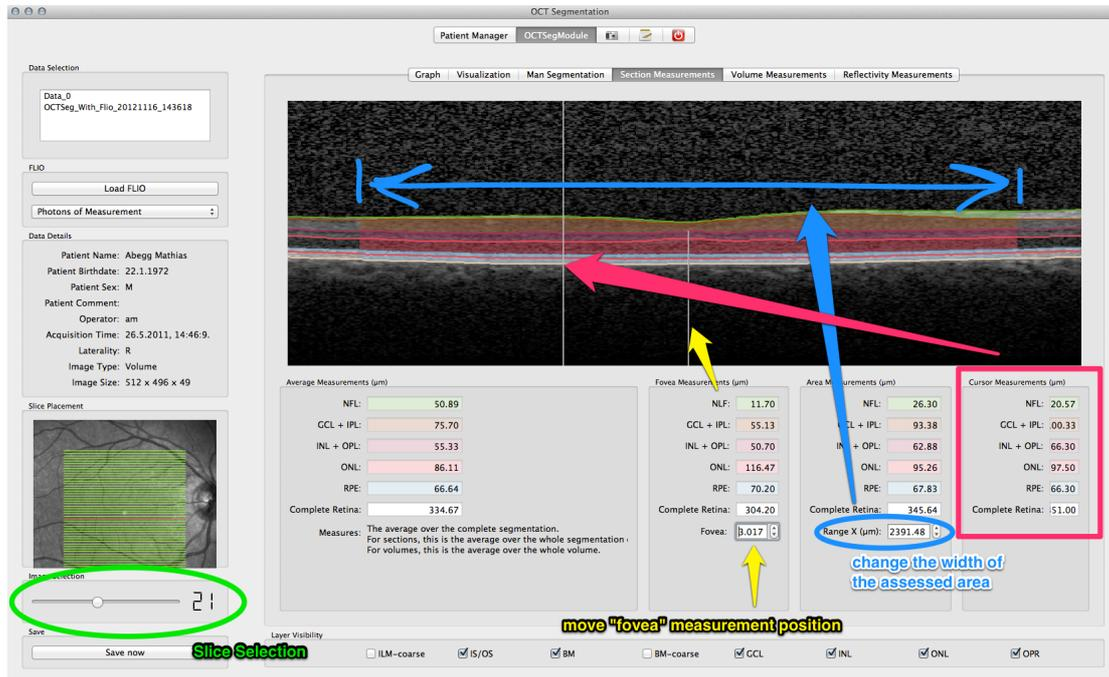
Figure 10: Section Measurement Screen
