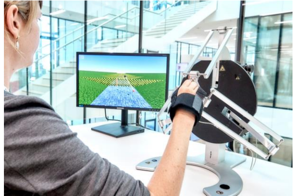
Figure 1: An example task designed, interacted via Delta.3 from Force Dimension.
