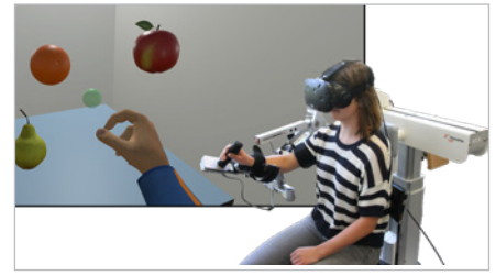
Fig. 4: Immersive VR to enhance neurorehabilitation. Virtual environment showing the avatar and three fruit types. The rehabilitation device is employed in a study with brain-injured patients.
