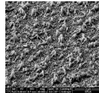
4 min oxygen plasma etched nanotexture PMMA resulting at 600 nm roughness
