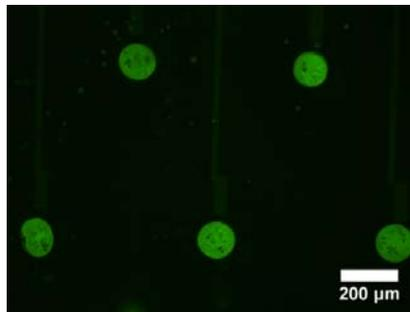
LIFT conditions: 10μM on donor, 300 mJ/cm<sup>2</sup>, Spot size: 50μm, 266 nm
