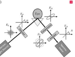
Rotating Compensator Ellipsometry Setup (a)
