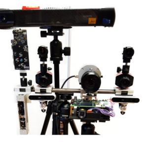
Test setup of different 3D measurement technologies and devices for the measurement of the human back
