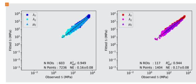
Linear regression between observed trabecular stiffness and predicted stiffness. Left: healthy controls. Right: OI.
