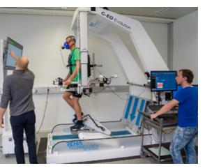
Cardiopulmonary rehabilitation with the G-EO System end-effector gait rehabilitation robot
