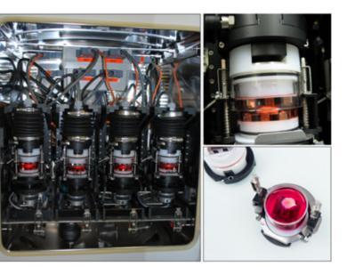
Specialized Bioreactor to apply compression and torsion for culturing culture under compression and torsion. Left inside incubator, upper right: close-up view of culture chamber, lower right: Inside view of culture chamber with positioned bovine coccygeal intervertebral disc. This device is worldwide unique.
