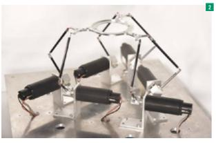
Robot with the end effector platform connected to six motors via legs.<sup>[12]</sup>
