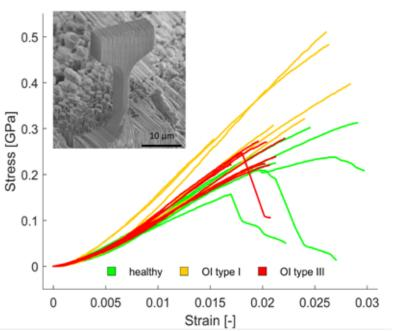
Stress-strain curve of micro-tensile specimen of OI and healthy control bone.
