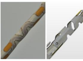
3D CAD design of a smart catheter with active transducers embedded (left) and prototype of a smart catheter with FEM-optimized LCP design for multiple passive electrodes
