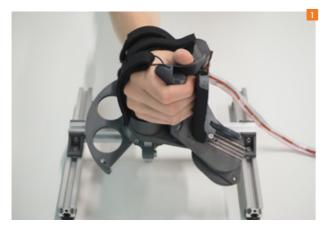
Prototype of haptic hand rehabilitation device for sensorimotor training after stroke
