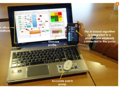
The Al-based algorithm, integrated into a highly secured Android smartphone, takes input from either a blood glucose meter or continuous glucose monitors, and outputs the daily insulin treatment. The algorithm learns while being used by the patient and is able to provide personalised advice on the insulin treatment.
