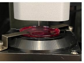
The mechanical properties of the cornea measured using instrumented indentation.
