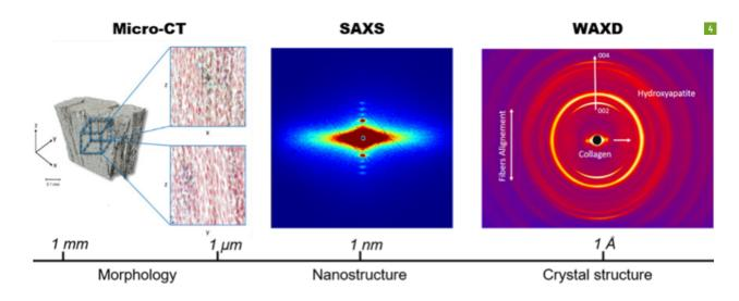
Holistic approach in the analysis of hierarchical structures: from morphology (mm-µm) over nanostructure (nm) to molecular structure (Å) using X-ray based methods.
