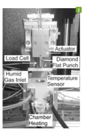
Micromechanical testing platform with the high strain rate and the temperature-controlling setup. The experiment chamber is heated with a heat exchanger that is fed with flowing water at a set temperature at the base of the chamber. The desired relative humidity is achieved by feeding a gas (usually air) with a controlled relative humidity into the chamber.
