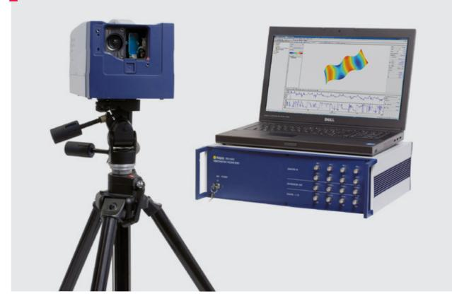
Laser Doppler Interferometer
