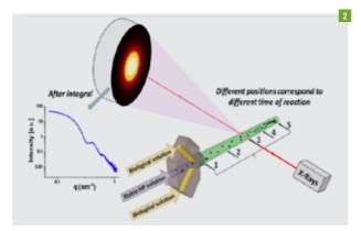
Scheme of the micro-fluidics SAXS setup for the in-situ investigation of early events in NPs' interations in a biological environment.
