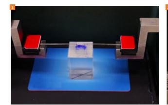
Corneal strips 150µm thick were cut into the cornea with a femtosecond laser to quantify the depth and orientation dependence of mechanical properties measured by a uniaxial tensile test.
