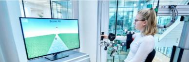
Virtual inverted pendulum task with ARMin exoskeleton robot
