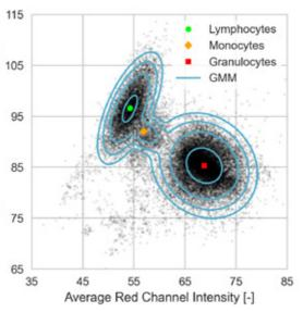
Scatterplot of cell-averaged red and green values of all WBC detected in 2 µL of blood that has flown through the microfluidic channel. Contour lines represent a three-component gaussian mixture model that are superimposed to determine the three major sub-types of WBC.
