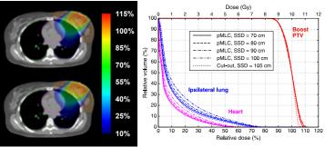
Dose distribution (left) and Dose Volume Histograms (right) of a 18 MeV electron treatment plan created for a left breast boost case.
