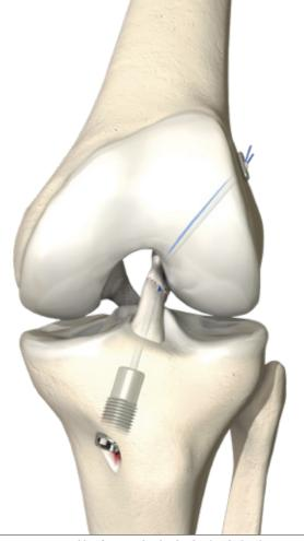
Sensor system capable of measuring in vivo loads wirelessly
