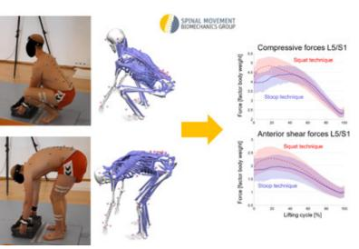
Simulating spinal loading using motion capture-driven musculoskeletal modelling
