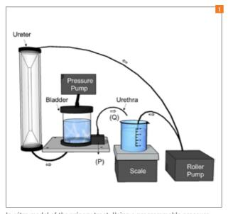
In-vitro model of the urinary tract. Using a programmable pressure pump, bladder pressure waveform and flow can be controlled to mimic physiological and pathological conditions.
