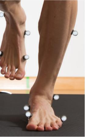
Clinically oriented measurement of foot kinematics by quantifying navicular bone motion using four reflective markers and 3D motion capture
