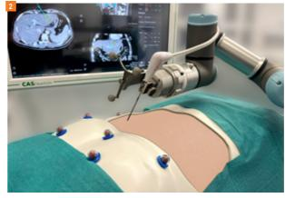
Prototype of a robotic system for thermal ablation.
