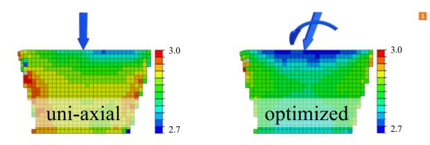
Standard uni-axial loading boundary conditions (left) and an optimized loading boundary condition (right).
