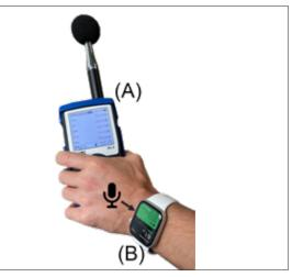
Noise monitoring using a sound level meter (A) and a smartwatch (B).
