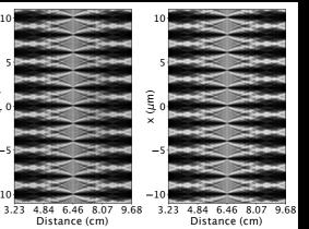
Talbot carpets obtained with Monte Carlo (left) and wave propagator (right) on the detector position x as a function of distance to the grating.
