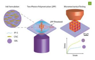
Overview of the 3D printing of microscale cellulose nanocrystalreinforced nanocomposites by two-photon polymerisation (2PP) and their micromechanical characterisation. Inks of GBL, CNC, and IP-S (left) were manufactured where three different CNC concentrations are used for the 3D micro-fabrication (middle). Their structuremechanical properties were determined by means of micro-compression (right) and Raman measurements.
