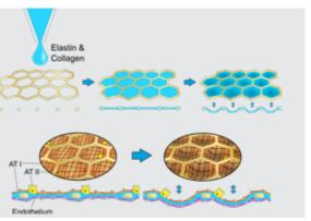
Concept of the second-generation lung-on-chip: a drop of collagen and elastin is pipetted on a thin hexagonal gold grid. The stretchable membrane is formed by surface tension forces and evaporation.
