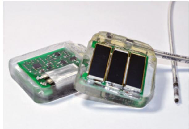
Testing of an implantable solar panel
