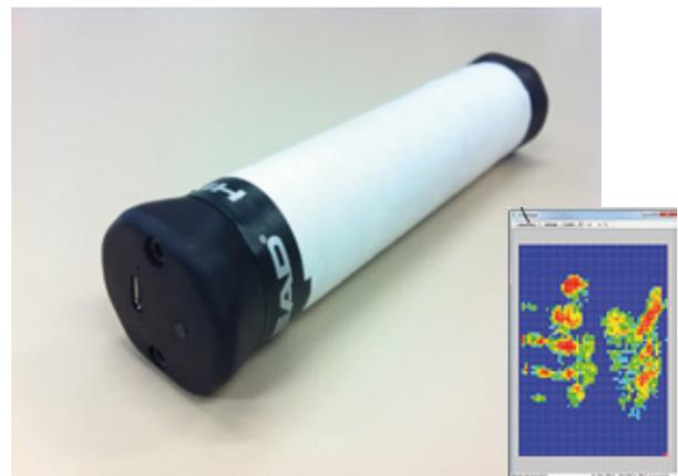
3000 pixels representing a hand imprint to be delivered in real time. This wireless device transmits data to a smartphone or another smart device for direct analysis. It can also be shared or stored. Data analysis algorithms have also been developed to facilitate the diagnosis. This project has been performed with EoSwiss Ltd. in Geneva. A patent application on this device has been submitted, and a clinical study is ongoing.
