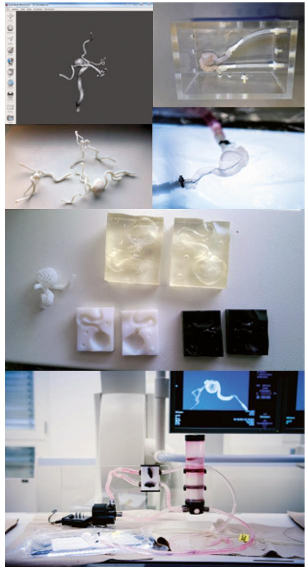
Developmental process of cerebral aneurysm models using additive manufacturing techniques (3D printing) based on patient specific 3D imaging data sets.
