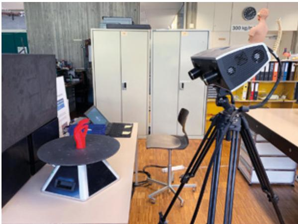
3D Scanner for rapid prototyping.
