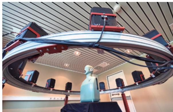
Multi-speaker set up for sound field audiometry
