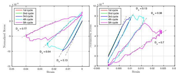
Cyclic normalised stress-strain curves for trabecular bone in compression and tension using explicit finite element analysis
