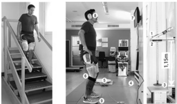
Left: Walking downstairs; Right: (1) electromagnet, (2) falling barbell weight, (3) stopper, (4) wire rope, (5) force transducer, (6) brace, (7) monitor for feedback, (8) headphones and attenuator, (9) force platform.
