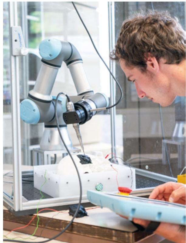
Cochlear implant surgery requires drilling near the facial nerve. The goal of the DrillMon project is to develop, optimize and characterize a system that combines a surgical drilling device with an electrical nerve stimulation probe. This allows surgeons to continuously monitor nerves while drilling with up to 80'000 rpm.
