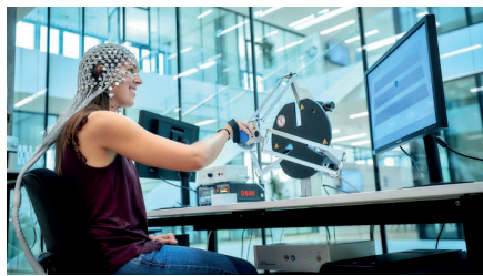
Fig. 2: Robotic somatosensory training with haptically rendered virtual textures.
