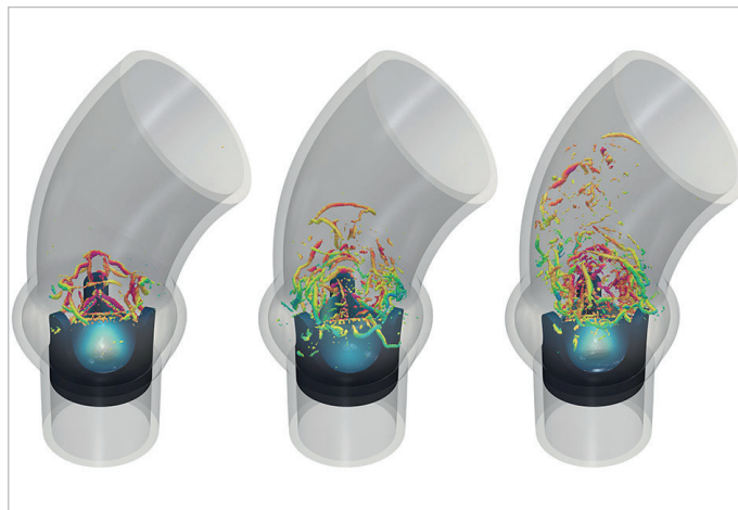
Fig 2: Microfluidic chip to model the blood flow in the heart muscle. Fig 3: Turbulent blood flow behind a heart valve prosthesis.
