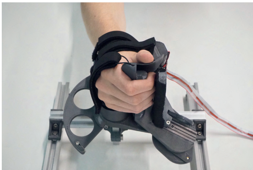
Fig. 1: Prototype of haptic hand rehabilitation device for sensorimotor training after stroke. Photo: Adrian Moser for ARTORG Center
