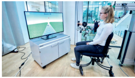
Fig. 3: Virtual inverted pendulum task with ARMin exoskeleton robot.
