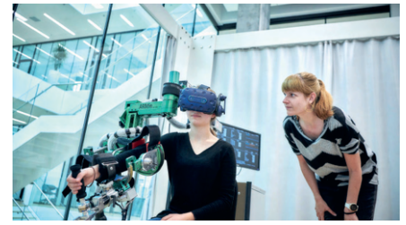
Fig. 4: Robotic motor training with ARMin exoskeleton in immersive virtual reality.
