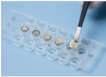
Fig. 2: Picture of the second-generation lung-on-chip with six wells with hexagonal gold grid.
