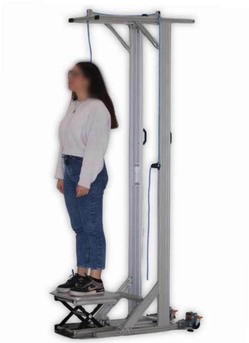
Fig. 1: A spinal suspension system was developed to measure spinal stiffness in adolescent idiopathic scoliosis patients.
