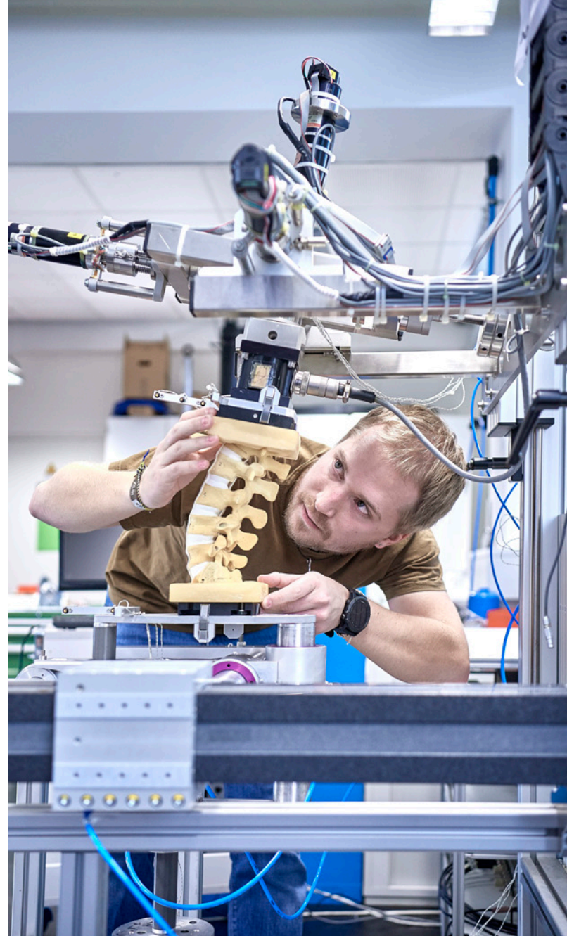
Evaluation of the intervertebral disc function: calibration of a spine testing system.
