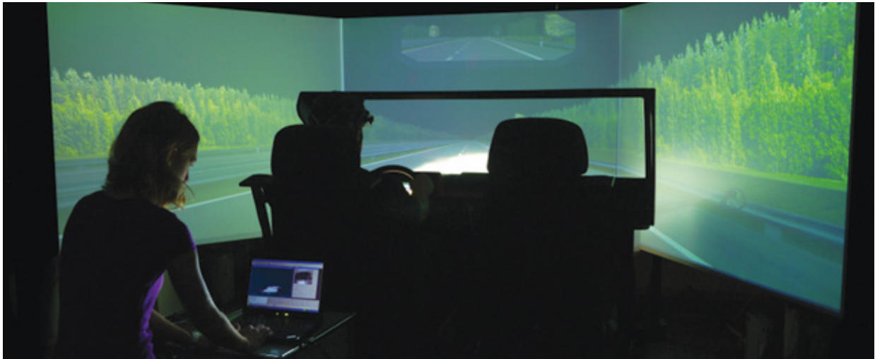
Simulated driving during a visual exploration experiment. The test subject wears a helmet with an integrated eye tracking camera to measure gaze direction.
