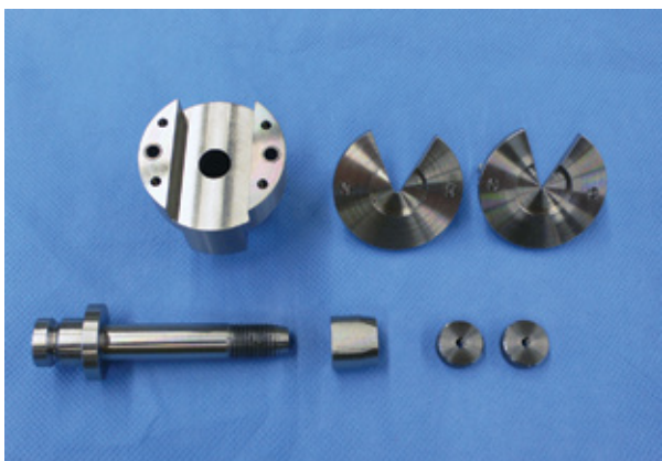
Components of the macro tensile test set up for testing of dental filling samples.
