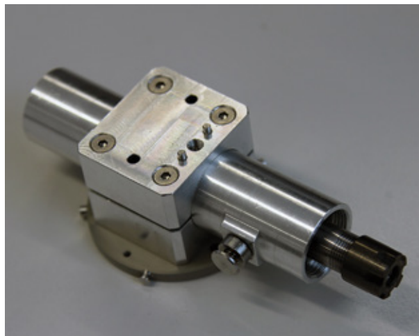
Custom drill hand piece for a minimally invasive robotic system.
