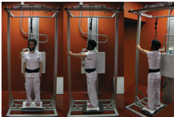
A spinal loading system has been designed to quantitatively assess the biomechanical properties of the patients' spine before scoliotic correction surgery.
