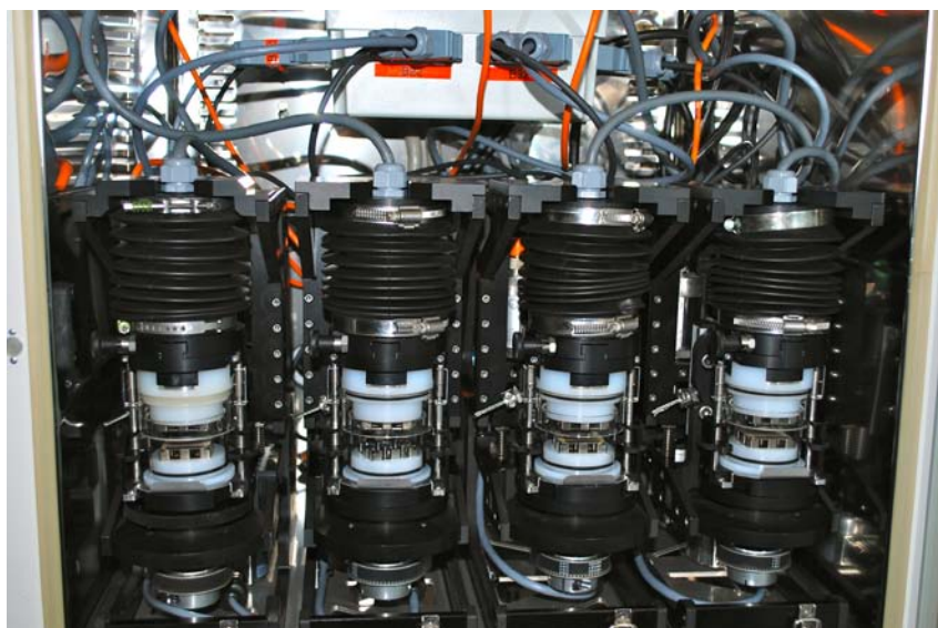
Two-degree of freedom loading device to culture bovine intervertebral discs under uni-axial compression and torsion. The device has been designed to be removed easily from the incubator unit and the entire set-up can be either force or way-controlled. A real-time processor unit is located outside of the incubator which is recording data and controlling the device.
